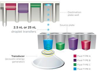
Acoustic droplet ejection - The transducer is positioned below the source microplate well and emits focused sound energy repeatably to the meniscus of the fluid to be transferred. A stream of 2.5 or 25 nL droplets (model dependent) is reliably ejected into a well of an inverted destination microplate
